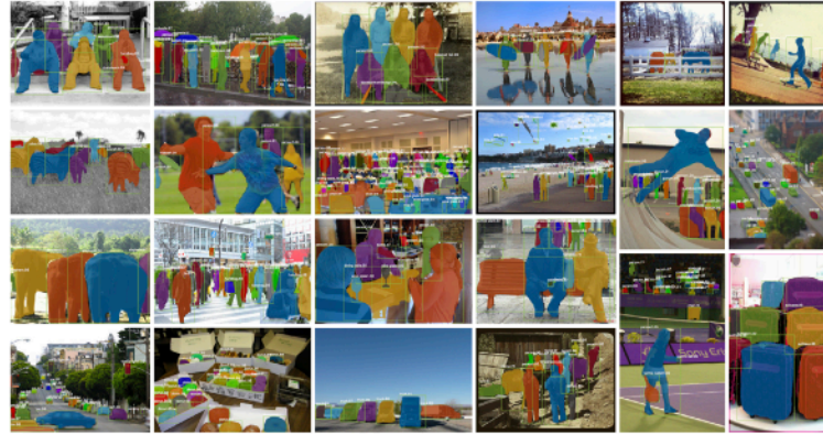
Figure 5. More results of Mask R-CNN on COCO test images, using ResNet-101-FPN and running at 5 fps, with 35.7 mask AP (Table 1).
